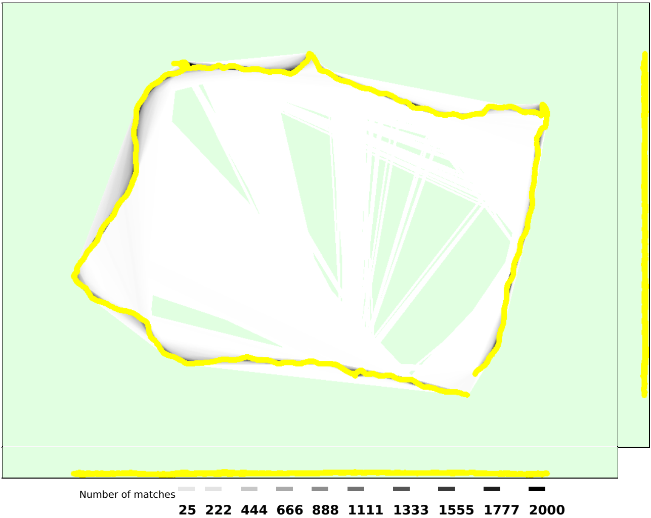
Figure 5: Computed image positions with links between matched images. The darkness of the links indicates the number of matched 2D keypoints between the images. Bright links indicate weak links and require manual tie points or more images.
