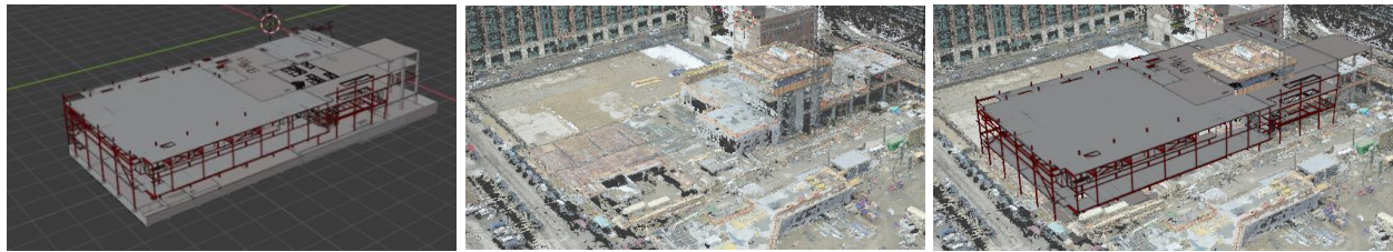
Figure 2. 4D as-planned BIM (left), 3D as-built point cloud model (middle), and finely registered as-planned and as-built model (right)
