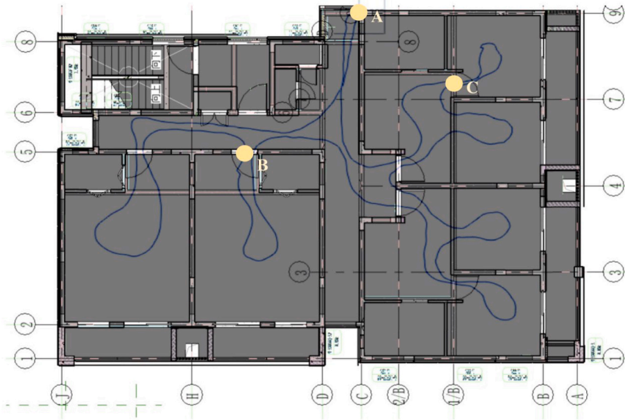
Fig. 10. Data collection diagram. Point A is the origin. Points B and C are two feature points with known true coordinates.
